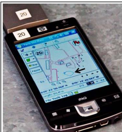
Figure 1. Field GIS Hewlett-Packard personal digital assistant with US GlobalSat GPS, and Farm Works field GIS software shown mapping a mosquito breeding pool identified by black arrow.
